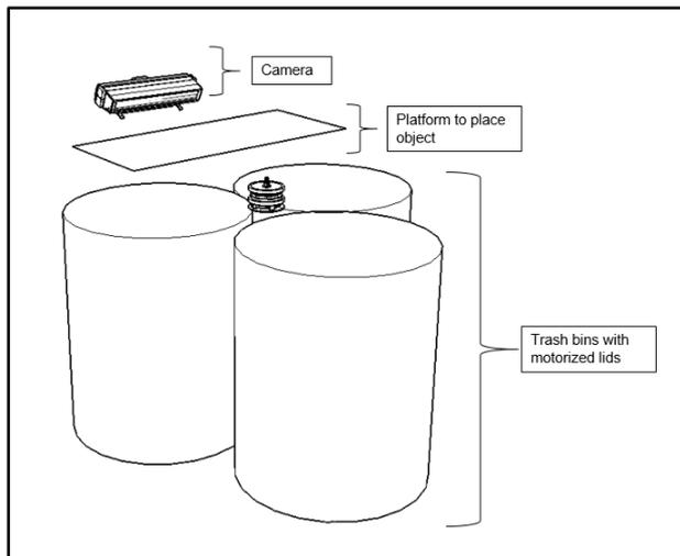
Figure 4: Manual Sorting with Classification
