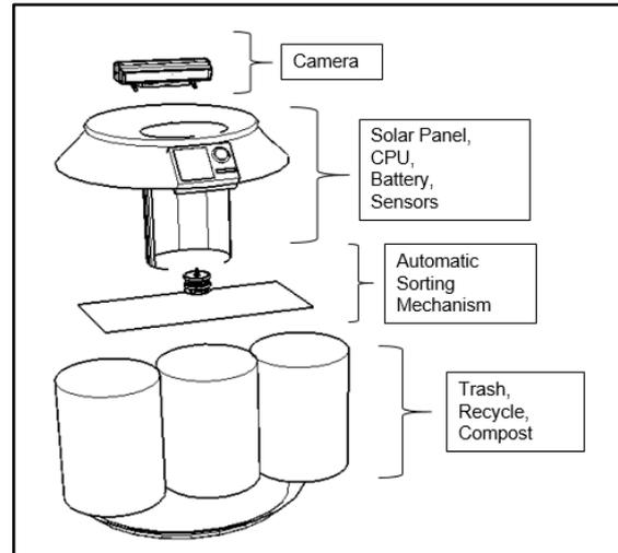
Figure 5: Automatic Sorting with Classification
